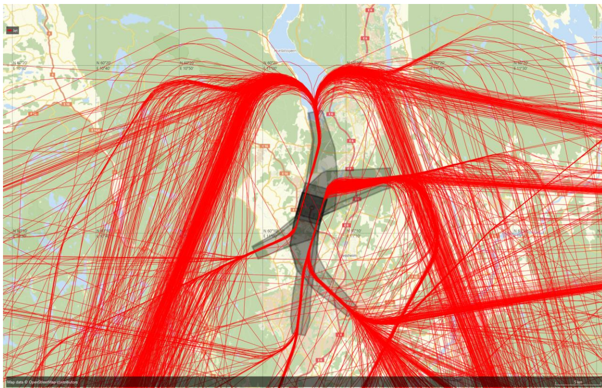
Figur 45. Avganger, Norwegian – Utland, Totalt 1734 flygninger B737-800 (1519), B737-800 MAX (215)
