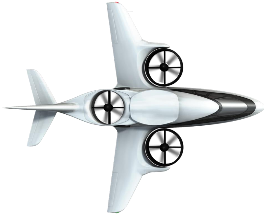
XTI aircraft, a 5-seater, hybrid electric VTOL plane utilizing the flexibility granted by electric motor propulsion (Credit: XTI Aircraft)
