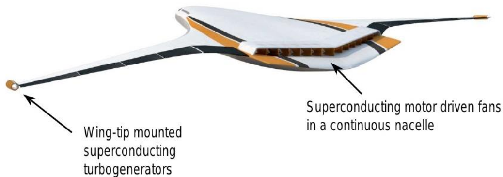
NASA CONCEPT: N3-X Distributed Turboelectric Propulsion System. (Credit: NASA)
