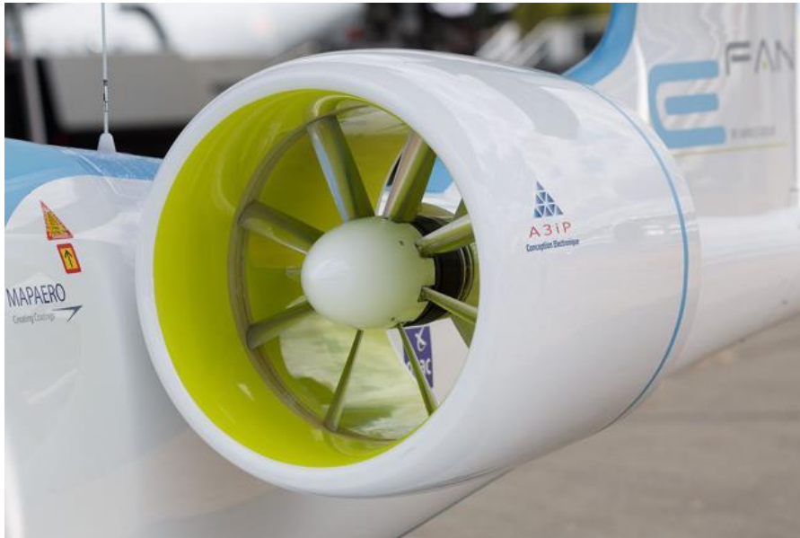
The Airbus E-Fan project used two ducted fan modules. (Credit: Airbus)
