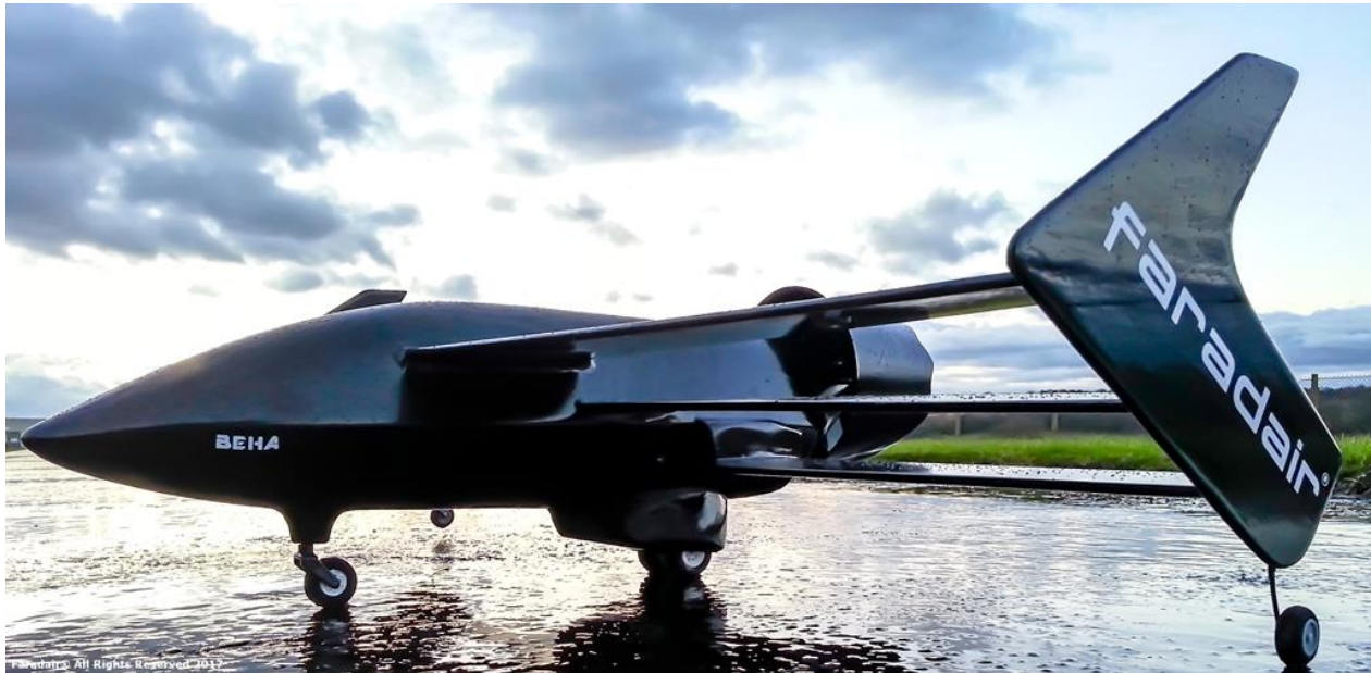
The Faradair BEHA (Bio-Electric-Hybrid-Aircraft), a 6-Seat aircraft with a Hybrid propulsion system. (Credit: Faradair)
