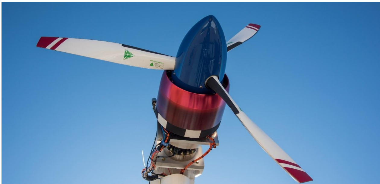
Electric engine with propeller seen on NASA's X-57 Maxwell's wingtip cruise motor/propeller. (Credit: NASA)
