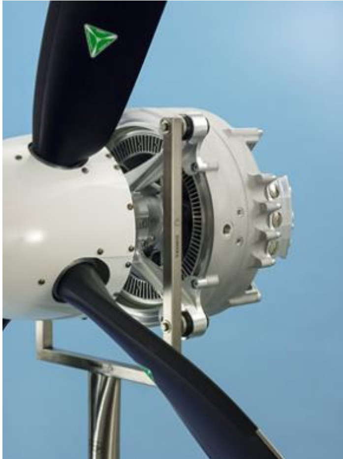
260 kw motor - 50 kg. (Credit: Siemens)
