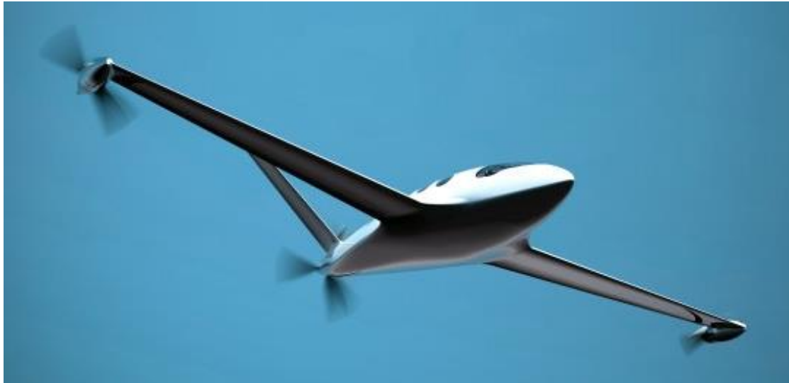
Eviation aims for a highly efficient composite aircraft with wing tip and tail electric propulsion. (Credit: Eviation)
